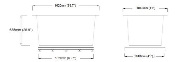
Do not scale drawing. Allow 110mm for air breather.
