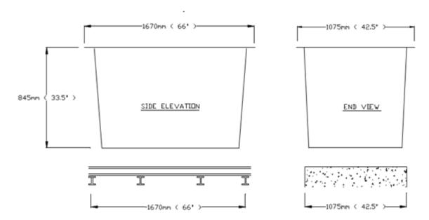
Do not scale drawing. Allow 110mm for air breather.
