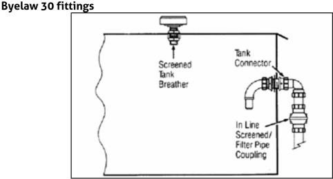
The overflows should be twice the cross section area of the inlet
